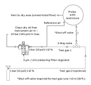
Fig. 8 Non-AutoCal with air as test gas 1
