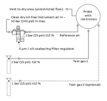
Fig. 7 AutoCal with 2 test gases
