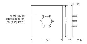
Standard mounting plate for 1.0 to 2 m (3.3 to 6.6 ft.) probes – Part No. AZ200 795  $\,$
