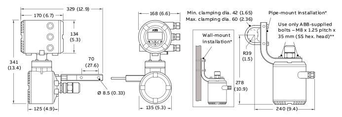
\*Wall- / Pipe-mount bracket plus U-bolt, pipe clamp and M8 fixings supplied as standard
