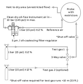
Fig. 9 Non-AutoCal with 2 test gases
