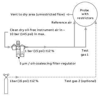
Fig. 6 AutoCal with air as test gas 1
