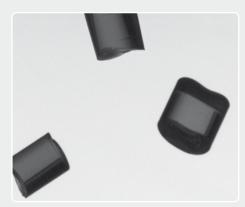
The advantage of the full-frame cameras used by the CAMSIZER P4 for the distortionfree recording of true particle projections is essential when measuring the particle shape.
