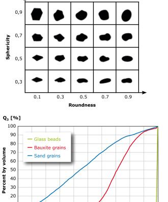
Chart for visual inspection of Roundness and Sphericity according to Krumbein and Sloss
