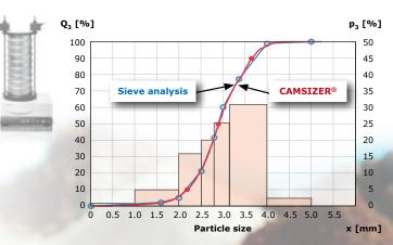
Perfect compliance of sieve analysis and CAMSIZER P4 measurement results for granulated fertilizer.
