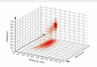
3D Cloud: Display of the 3 independent analysis parameters size, transparency, and aspect ratio for a mixture of road marking materials consisting of irregular shaped, non-transparent antiskid aggregates and round, transparent glass beads.
