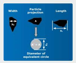
Examples of size parameters from the analysis of individual particle images derived from the high resolution scans of the CAMSIZER P4.
