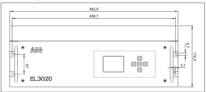
Only the front view of the housing (with its height differing from the standard dimension) is depicted in this dimensional drawing. Note: Refer to the dimensional drawing on page 33 for other views and dimensions of the housing.
