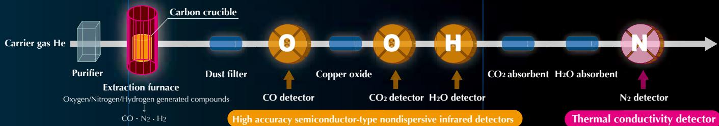
■ Oxygen determination : 2 NDIR detectors for high accuracy among the full measurement range. Automatically controlled by the software.
