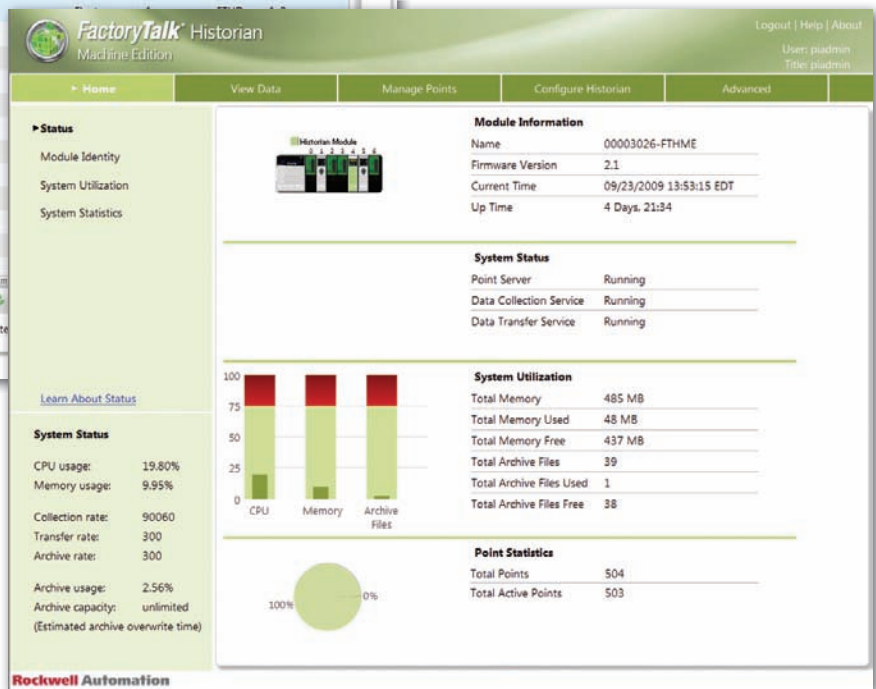
The FactoryTalk Historian ME home page give a quick and clear overview of module status.
