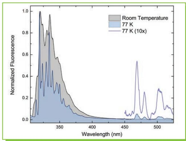
Temperature can add thermal broadening to fluorescence spectra and increase phosphorescence quenching. Spectra of Naphthalene dissolved in Methanol measured at room temperature (298 K) and in a liquid nitrogen dewar accessory (77 K). The low temperature spectrum reveals rich vibrational structure and longer wavelength phosphorescence. Phosphorescence peaks are also shown magnified 10x for clarity.
