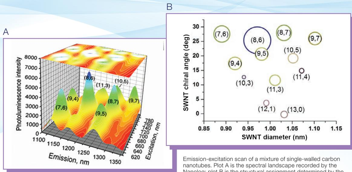
Emission-excitation scan of a mixture of single-walled carbon nanotubes. Plot A is the spectral landscape recorded by the Nanolog; plot B is the structural assignment determined by the Nanosizer software. Diameters and colors of circles in plot B are related to peak-intensities in plot A.
