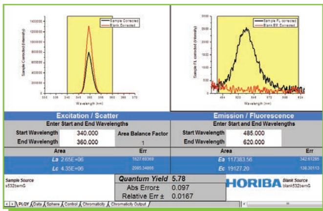
High precision absolute quantum yield characterization of a quantum dot sample enabled by the Quanta-φ integrating sphere accessory.
