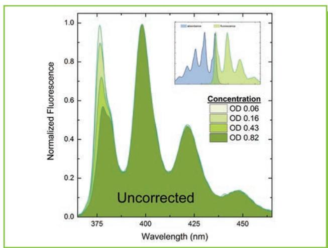
Reabsorption of fluorescence photons can occur even at moderate concentrations, and lead to increasing distortion of spectra with increasing concentration (left). The Fluorolog-3 software can correct this phenomenon, (known as the inner-filter effect), using the sample absorbance measured by the absorbance accessory (right).
