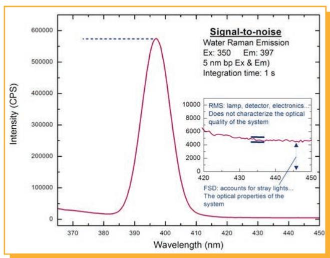
The Raman band of ultra-pure water was measured in a standard 1 cm quartz cuvette. HORIBA qualifies its instruments with two measures of signal-to-noise: Root Mean Square (RMS) and First Standard Deviation (FSD) of light from its standard Xenon lamp source.
