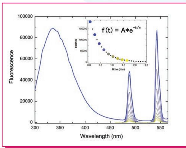
Complex solutions like this mixture of Bovine Serum Albumin (BSA) and Terbium Chloride ( $Tb^{3+}$ ) can be challenging to interpret. Using the pulsed light source of the phosphorescence option allows you to temporally “gate out” the BSA fluorescence, leaving only the  $Tb^{3+}$  phosphorescence. Inset shows the single wavelength phosphorescence decay of  $Tb^{3+}$  in this mixture; colored circles correspond to the gated spectra in the main figure.
