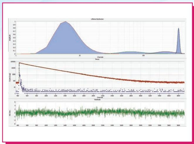
Non-extensive distribution fits: 1,8-ANS exists in free solution and partitions into several disparate environments in Bovine Serum Albumin. Within each environment, a distribution of states exists with a corresponding distribution of lifetimes. Fluorolog-3 software not only offers standard discrete exponential fits, but also several energy transfer and distribution models, including the proprietary non-extensive distribution shown here.
