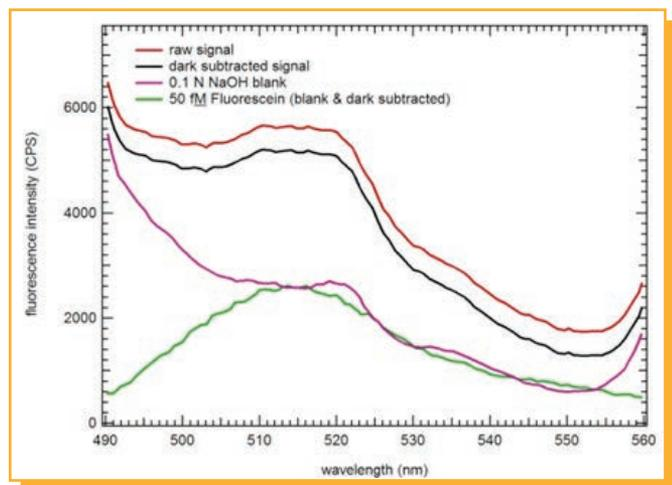
50 fM Fluorescein in 0.01 N NaOH. Subtracting the dark counts and the signal from the solvent alone reveals the clean Fluorescein spectrum at ultra-low concentration.
