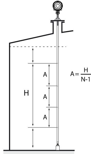
Recommended temperature sensor positions for custody transfer according to API. Example: 4 spot elements, H=9. A=3 m
