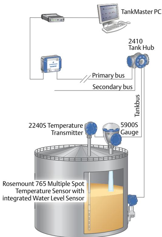
Rosemount 765 Multiple Spot Temperature Sensor installed together with a Rosemount 2240S Multi-input Temperature Transmitter, in a Tank Gauging System
