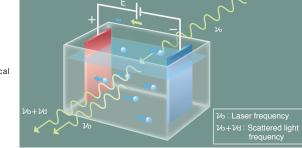
$\zeta$ :Zeta potential U:Electrical mobility E:Electric field strength n:Solvent refraction index  $\epsilon$ :Solvent dielectric constant  $\eta$ :Solvent viscosity  $f(\kappa a)$ :Henry coefficient
