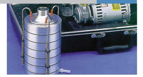
The Thermo Scientific Six Stage Viable Andersen Cascade Impactor (ACI) is a bioaerosol and microbial particle sizing sampler designed to measure the concentration and particle size distribution of aerobic bacteria and fungi in intramural or ambient air. All particles collected, regardless of size, shape or density are aerodynamically sized and can be directly related to human lung deposition.
