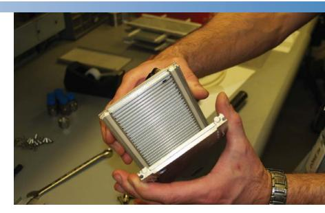
The Thermo Scientific Particulate Dryer Maintenance Program helps to protect your instrument from particulate overload. To ensure peak-performance of the Thermo Scientific TEOM 1405-F, TEOM 1405-DF and the Model 8500-C, it is recommended that the dryer be serviced every 12 months or as often as required.
