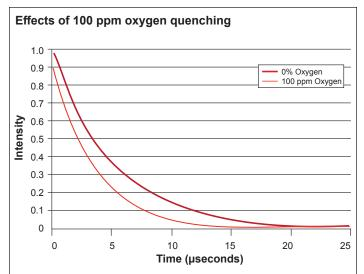
The affect of oxygen quenching on light intensity from the luminophore sensor is shown above. Light emitted from the excited luminophore has higher intensity over a longer time period than when oxygen is present. The intensity and time are measured by the spectrometer within the OXYvisor to provide an oxygen measurement.
