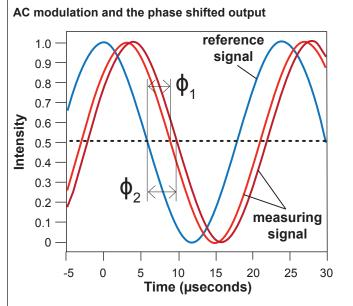
AC modulation of the blue light results in a similar waveform of the emitted red light from the luminophore sensor. The presence of oxygen causes a phase shift between  $\Phi_1$  and  $\Phi_2$  of the red light waveform. Measurement of this phase shift proportionally matches the loss of intensity shown in figure 2 above. The combination of both measurement techniques provides a stable, accurate method to measure oxygen in liquid and gas phase applications.
