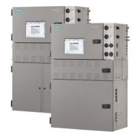
Special analytical tasks require stable temperatures in the oven to optimize separating performance of the components. The requirements for optimum separation performance are met with our two oven types. The airless oven provides extremely stable isothermal temperatures with high control accuracy, completely without the use of air. The airbath oven offers both isothermal and temperature-programmed operation with air supply.
